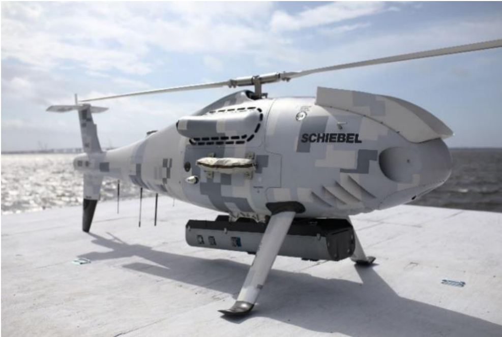
Figure 4. Fugro RAMMS installed on UAS.
