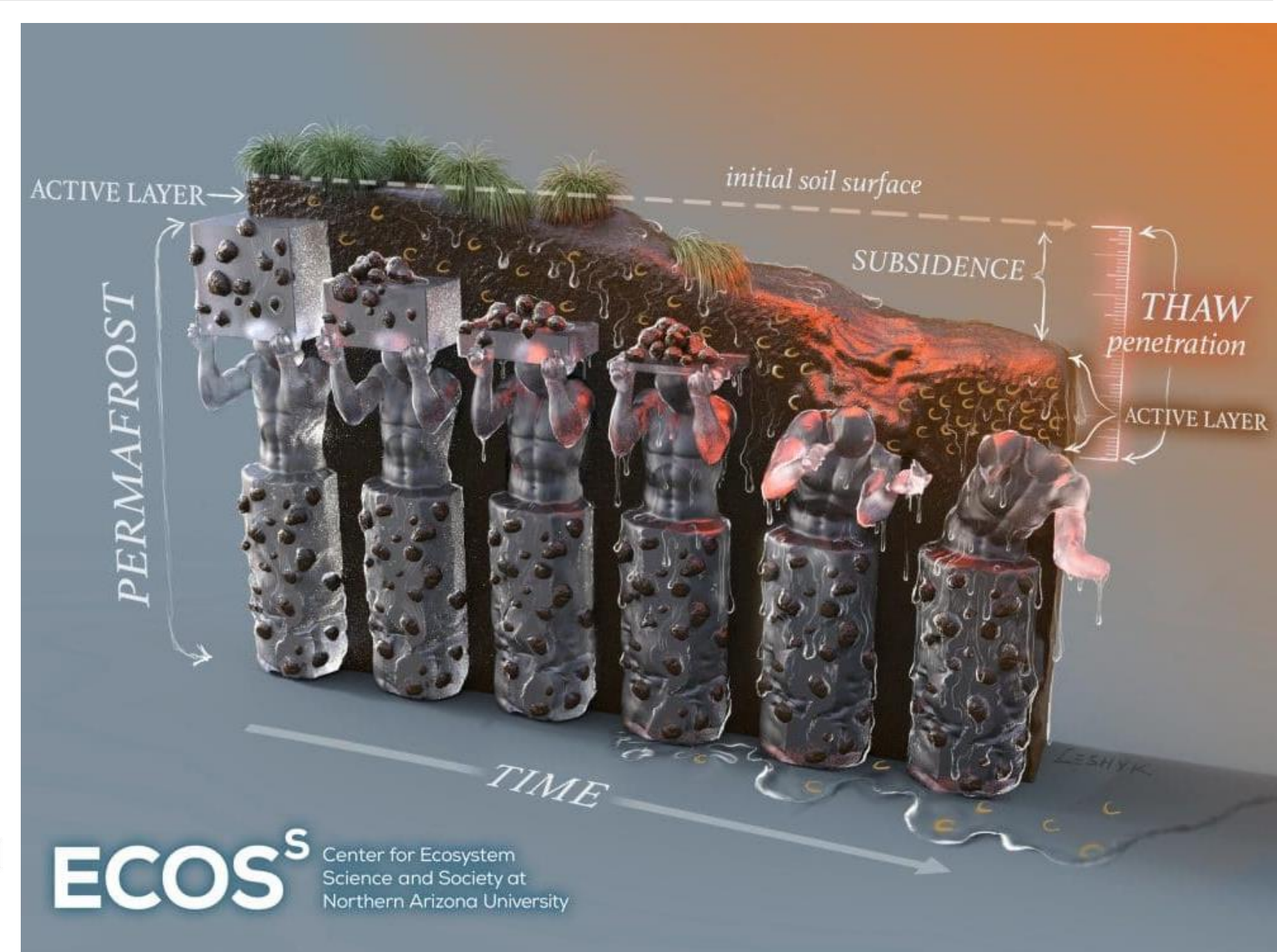
Figure 4. Thawing permafrost may lead to ground subsidence as a result of thaw settlement due to phase change from ice to water and the loss of melted water draining away from the ground. Ground settlement from thawing permafrost is a major hazard for stability and safety of infrastructure (Ma et al., 2012), resulting in increased maintenance costs and remediation work to ensure structural integrity (Osterkamp & Burn, 2003). Image Credit: Leshyk, V.O. Center for Ecosystem Science and Society, Northern Arizona University ( https://www2.nau.edu/schuurlab-p/ ).
