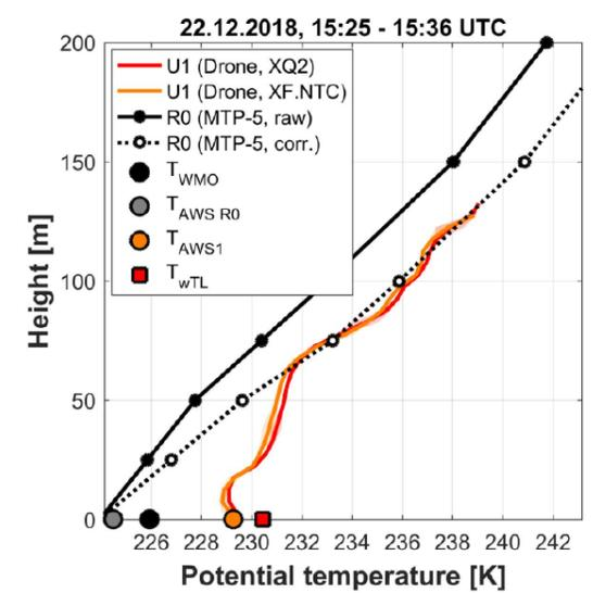
FIG 2. Vertical profiles of potential temperature obtained by drones (colored) in urban areas and the temperature profiler MTP-5 (b/w) at the airport, Nadym, Russia. Dots shows temperature at 2 m meters from relevant automated weather stations (AWSs).
