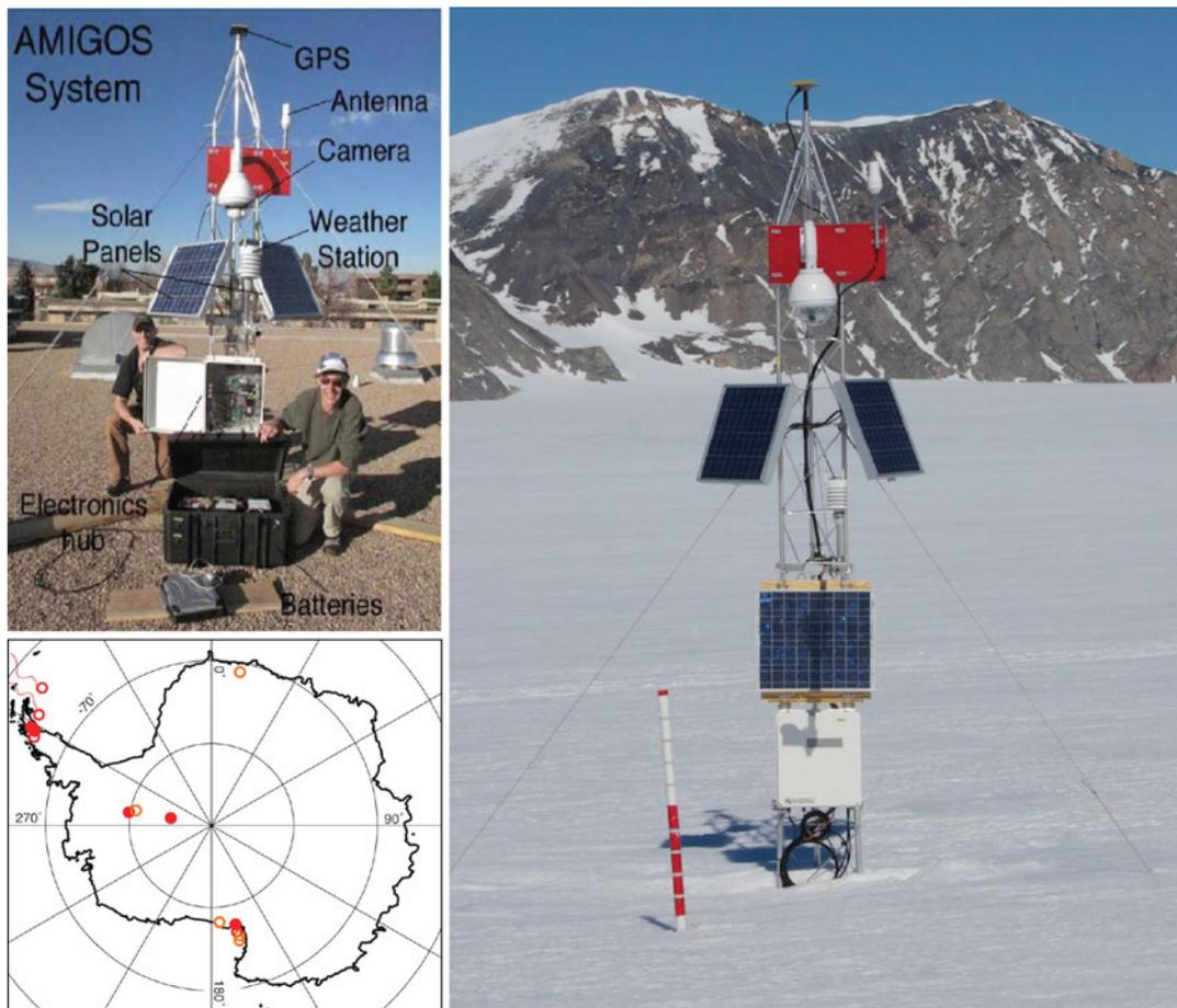
Figure 1. Current AMIGOS system configuration (top left and right side), and installation sites (lower left).
