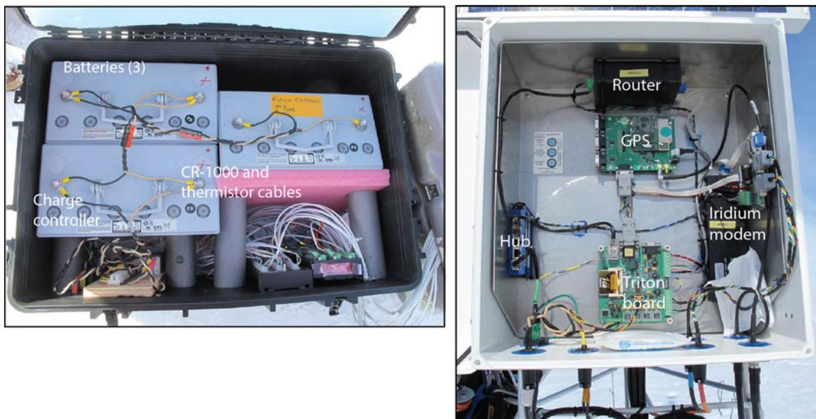
Figure 2. View of main electronics enclosure (right) and battery box (left).
