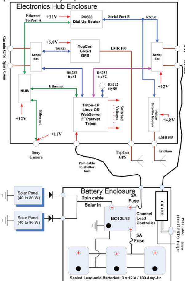
Figure 3. Block diagram and description of current AMIGOS configuration and components.
