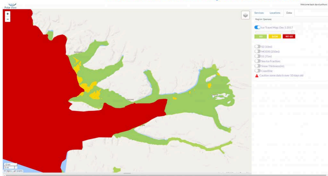
Figure 3. The community ice information service uses near-real-time Sentinel 1 satellite imagery to monitor the ice conditions for communities, offering 'go', 'slow go' or 'no go' recommendations using a green, yellow, and red colour code. Also included is a selection of satellite images (Sentinel 1 and 2, and Modis), locations of interest, a community base map containing local knowledge, information from the Copernicus marine service. http://floedge.polarview.org
